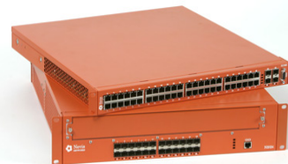
The two form factors of the Nevis security appliance are shown: The 48-port LANenforcer 1048 secure switch (top), and the LANenforcer 2024/2124 security appliance.
